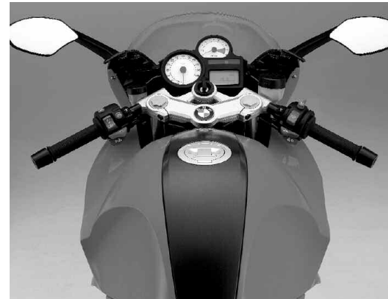
Instrumentation includes a large analog-type speedo (left) and tach (top) together with the usual information display. The mirrors are good, but not as wide as they might be, and the handlebars, although they look low, are close and comfortable.
