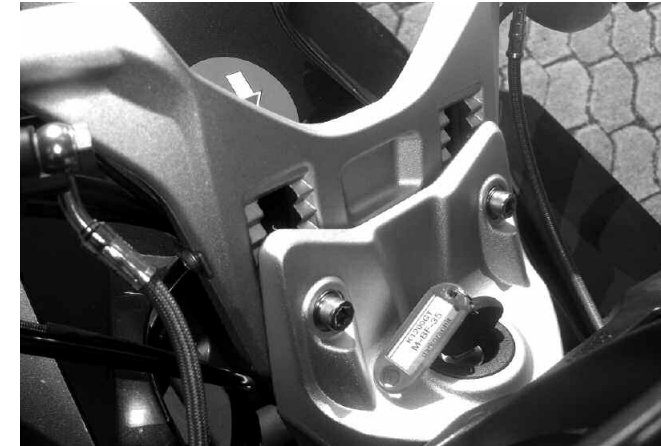
The handlebar mounting allows four positions and is angled so the bars move away as they go lower. Note the braided stainless brake/clutch lines.
