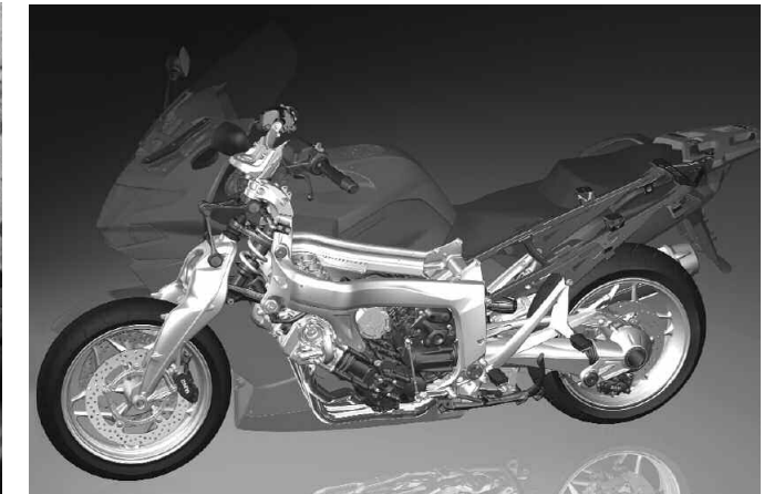
A look beneath the skin of the K1200GT reveals the high-tech alloy chassis and advanced suspension shared by the K1200S and R-models.
