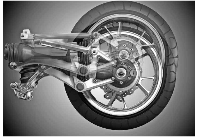
Above: The maximum travel of the Tetralever shaft drive system and the Uni-Trak rear suspension are shown. The linkage is double sided for strength, necessary with the engine's power. It rides just like a chain-driven bike, with no odd lift or squat.
