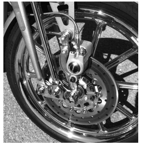
The Springer is the only model in H-D's lineup to use the old single-piston high-effort front brakes.
