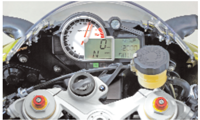
The attractive dash layout features a shift light next to the tach.
