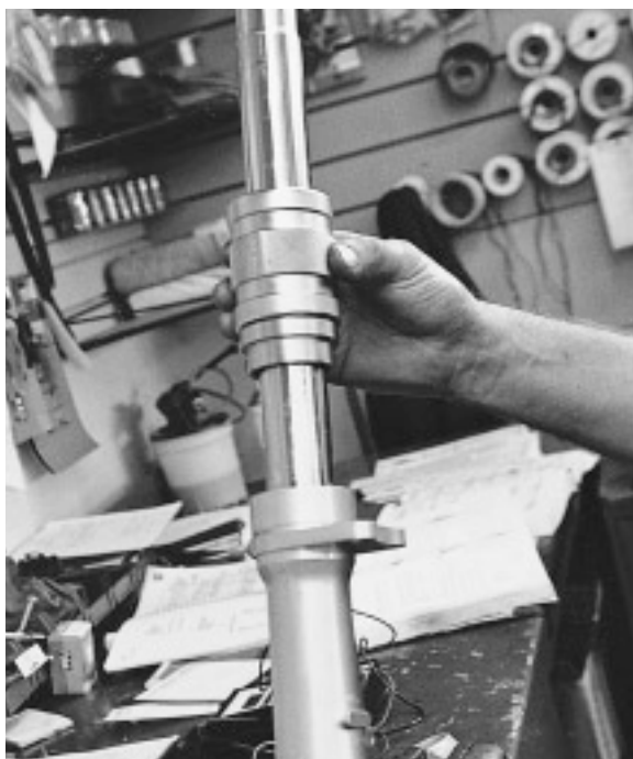
Left —Oil seals should be installed with a special “driver” made specifically to fit your make and model motorcycle. Any twisting, binding or uneven pressure on the seal during installation will virtually ensure reduced service life, if not result in almost immediate seal failure. Right —Even though the exact amount of carefully measured fluid was installed with reassembly, you should double-check the levels by measuring from the tops of the tubes with the forks fully compressed.
