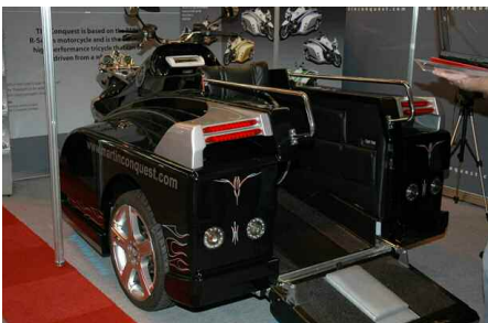
Left and Center: Making its first public appearance, and designed and built in the UK by Martin Conquest Ltd, the "Conquest" is a trike with BMW R1150R steering and power, able to accommodate a rider in a wheelchair, complete with an easy access automatic ramp at the rear. The vehicle comes with a six speed gearbox plus reverse, and has an unbelievable amount of optional equipment available—from Xenon headlights to parking sensors and even Sat Nav. Deliveries will begin in Spring 2006. Right: Ducati's 2006 ST3s ABS, now replacing the ST4s, the 6-valve motor now with new ignition and injection systems, plus "auto idle speed control" adds up to the Euro 3 emission standards of 2007, they don't come any cleaner than this one.
