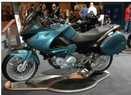
Left: The Honda Deauville continues in the 2006 line, and now comes with ABS and subtle restyling. Growing in popularity with the touring brigade, its 680cc 52°, 8-valve, V-twin is now punching out 65 hp @ 8000 rpm. Weight is 481lbs. Center: Honda's new CBF1000F/ABS, a well balanced looking machine, the 998cc DOHC 16-valver producing 101 hp @ 8000 rpm. Right: CCM are busy extending their 2006 range including this new FT35 model being unveiled by Nick Jeffries left and Niall Mackenzie.
