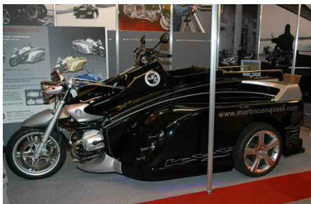
Left and Center: Making its first public appearance, and designed and built in the UK by Martin Conquest Ltd, the "Conquest" is a trike with BMW R1150R steering and power, able to accommodate a rider in a wheelchair, complete with an easy access automatic ramp at the rear. The vehicle comes with a six speed gearbox plus reverse, and has an unbelievable amount of optional equipment available—from Xenon headlights to parking sensors and even Sat Nav. Deliveries will begin in Spring 2006. Right: Ducati's 2006 ST3s ABS, now replacing the ST4s, the 6-valve motor now with new ignition and injection systems, plus "auto idle speed control" adds up to the Euro 3 emission standards of 2007, they don't come any cleaner than this one.
