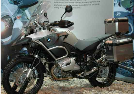
Left and Center: Debut of BMW’s latest model, the R1200GS Adventure, shown fully equipped and now offered with a wider range of special equipment than the old R1150GS. Output of the 1170cc twin is a straight 100 hp @ 7000 rpm, with six-speed transmission. BMS-K EFI is used plus a three-way catalytic converter, while the tank capacity is 8.7 gallons and dry weight 492 lbs., wet it rises to 564lbs. Right: The F650GS to be used in the next Dakar by Charlie Boorman, with much of the specialist Dakar kit from Touratech, it appears to be ready to go except for sponsor stickers.
