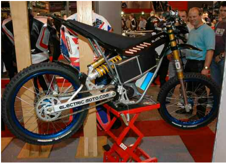
Left: A real novelty at Birmingham was this “Blade T6”—an electric dual-purpose lightweight motorcycle of high quality. Designed we are told by US and European engineers, it was inspired by moto-cross, trials, mountain biking etc. Frame is Laser cut tube, and suspension the best—from Ohlins, producing 25.7 hp the T6 accelerates from 0 to 30 mph in 4.1 seconds with a top speed of 40 mph. Go anywhere in silence, that’s for sure. Center and Right: Arlen Ness had a handful of exotic custom bikes on show, this one has a pair of 1000cc Sportster motors to move it.
