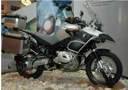
Left and Center: Debut of BMW’s latest model, the R1200GS Adventure, shown fully equipped and now offered with a wider range of special equipment than the old R1150GS. Output of the 1170cc twin is a straight 100 hp @ 7000 rpm, with six-speed transmission. BMS-K EFI is used plus a three-way catalytic converter, while the tank capacity is 8.7 gallons and dry weight 492 lbs., wet it rises to 564lbs. Right: The F650GS to be used in the next Dakar by Charlie Boorman, with much of the specialist Dakar kit from Touratech, it appears to be ready to go except for sponsor stickers.
