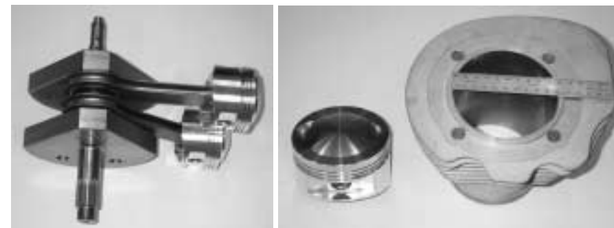
Left: Crank assembly with H-beam connecting rods and JE pistons. Right: 100mm piston and cylinder assembly.
