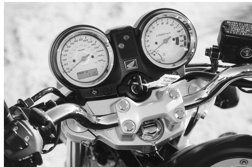
Above: The 599 offers no real wind protection, a serious drawback, if high speeds are part of your everyday riding. And, although the instrumentation looks basic, it is complete and very readable. Note the rectangular backbone tube connecting to the steering head, basic but effective.
