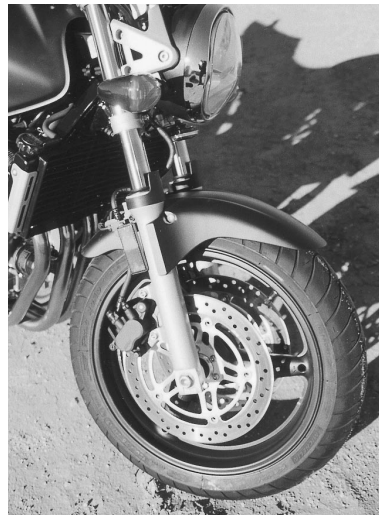
Above: The two-piston front brakes stop very well and give good control feel but suffered from chatter during testing.
