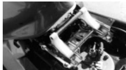
Above: Seat adjustment mechanism allows three positions, from 30.5" to 31.75".
