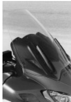
Above: The electrically adjustable windshield in its lowest and highest positions. Another 60mm of height is possible by repositioning the shield on its mounts, which requires removing four screws, and is the only adjustment provided on the Standard Model ST1300. We found the new headlights very attractive.
