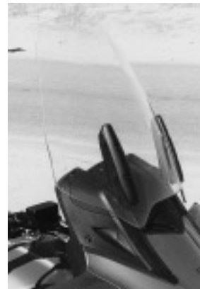
Above: The electrically adjustable windshield in its lowest and highest positions. Another 60mm of height is possible by repositioning the shield on its mounts, which requires removing four screws, and is the only adjustment provided on the Standard Model ST1300. We found the new headlights very attractive.
