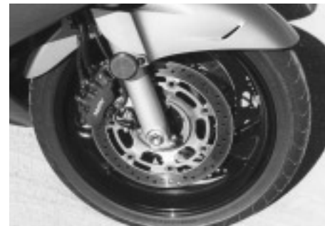
Below: The brakes are much more powerful than the ST1100's but we found the brake pads almost too progressive. The Linked Braking System is carried over, but with less "bias" than before.
