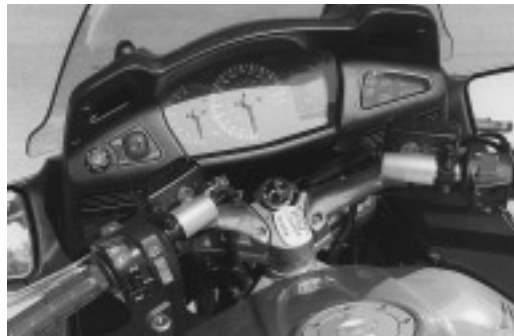
Left: The speed and tach are easy to read, but the LCD displays aren't. Note the lower surface of the dash, which looks to be ready for speakers. The knob on the left top adjusts headlight aim, and the button next to it toggles through the various settings and resets.
