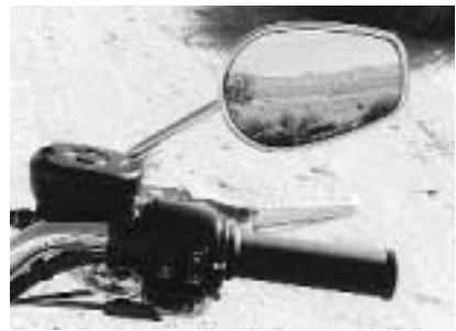
Below: The mirrors now have longer stalks to greatly improve the rear view. Smaller, 1 1/2" handgrips fit smaller hands and reduce the reach to the levers.
